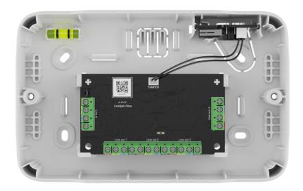
LineSplit is designed for indoor installation only. It is recommended to install device into Case. The casing is available in multiple versions. Installing one LineSplit module or <u>several devices</u> into Case is possible. Use <u>Case configurator</u> to get the most optimal placement of your Fibra devices in the casing.
