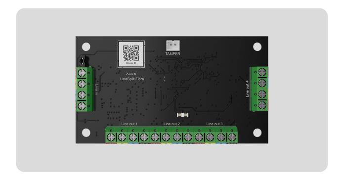
**Superior LineSplit Fibra** is a module designed to split one Fibra line into four ones. Each device output line can have a length of up to 2,000 meters when connected using the U/UTP cat.5 twisted pair cable. LineSplit can be installed at any point of the line, in particular after another LineSplit.
