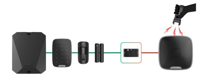
You need to connect one input and one output Fibra line to LineProtect. Use **Superior LineSplit Fibra** to divide the line. Do not install LineProtect on the Fibra line created in a **Ring** topology.
