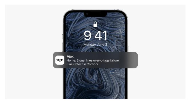
Fuses are triggered if an abnormal voltage is supplied on the Fibra line. In this case, LineProtect can fail, so it needs to be replaced. The users and the security company will receive the corresponding notification.
