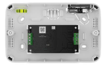
We recommend installing LineProtect into Case. The casing is sold separately and available in multiple versions. Installing a single module, several modules, or several other devices into Case is possible.
