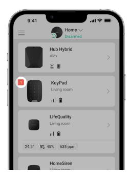
If a keypad malfunction is detected, a malfunction counter is displayed in Ajax apps in the upper left corner of the device icon.
