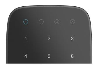
Superior KeyPad Fibra can report the current security mode, button pressings, malfunctions, and other conditions with LED indication and a sound signal.
