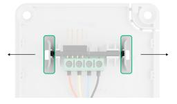
**3.** Prepare holes for cable output in advance. To output cables from the back of the keypad, break out the perforated part on the SmartBracket mounting panel. To output cables from the bottom of the keypad, make holes in the bottom of the enclosure using a drill bit, a special
