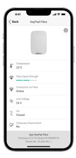
The states include information about the device and its operating parameters. The states of Superior KeyPad Fibra can be found in the Ajax app:
