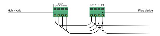
For the **Beam** (**Radial**) topology, be sure to install a 120 Ohm terminating resistor at the end of the line (included in the hub complete set). The terminating resistor is connected to the signal terminals of the last detector on the line.
