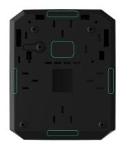
2. Secure the casing on the vertical surface at the selected installation location with the bundled screws using all fixation points. One of them is in the perforated part above the tamper — it is required for tamper triggering in case of any attempt to detach the hub casing.
