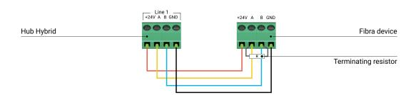
With the **Ring topology**, a terminating resistor is not needed. In this case, connect the last device in the line to the next Fibra line of the hub.
