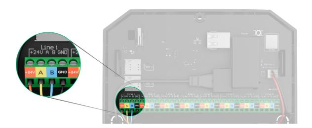
Superior Hub Hybrid (2G) / (4G) has 8 Fibra lines. Numbers from 1 to 8 are indicated on the control panel board.
