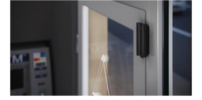
If the window has a ventilation mode, the detector should be installed on the upper part of the window. Otherwise, when the window is opened for ventilation, the detector gets closer to its own magnet and may perceive it as an attempt to mask it. To avoid false alarms, install the detector on the upper part of the window.
