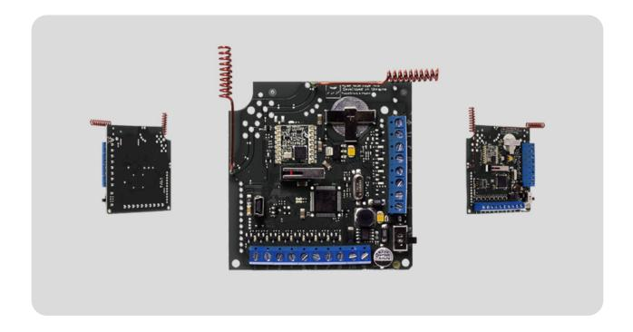
Wireless sensors' receiver **ocBridge Plus** is designated for connecting compatible Ajax devices to any third party wired central unit (panel) with a help of NC/NO contacts. Ajax system has two-way connection with the sensors which enables it's functioning in two modes: active mode and passive mode. When the system is in passive mode, wireless sensors switch to power-saving mode, which makes it possible to extend significantly battery life.
