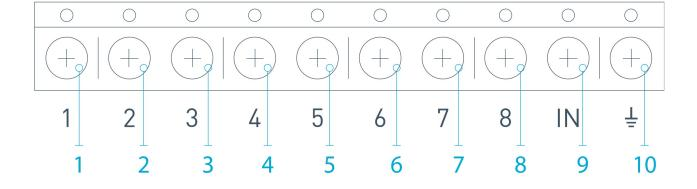
Other 5 outputs of ocBridge Plus are service zones and correspond to the service inputs of the alarm system central unit.
