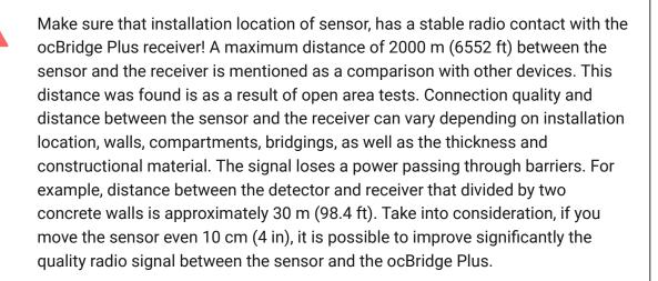
5. Select an appropriate place to install the sensors.
